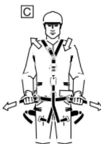
C. Adjust the belt strap. Always protect free ends of the straps with the loops. Adjust the shoulder straps.
