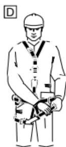
D. Fasten and adjust thigh straps. Always protect free ends of the straps with the loops.
