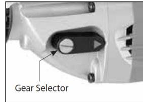
Pop the Gear Selector Tab out of the detent then slide the selector back for low or forward for high to change the gear. It may be necessary to turn the spindle slightly in order for the gear to be engaged. Once engaged, pop the tab into its detent.
